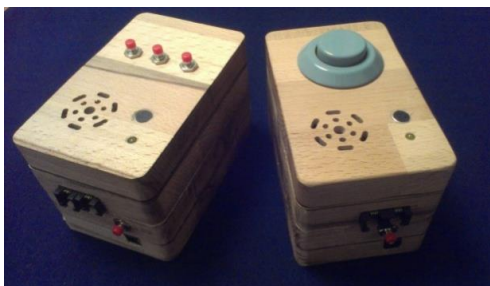
Figure 3. Final design of the device, two interface versions: buttons and rotational knob
